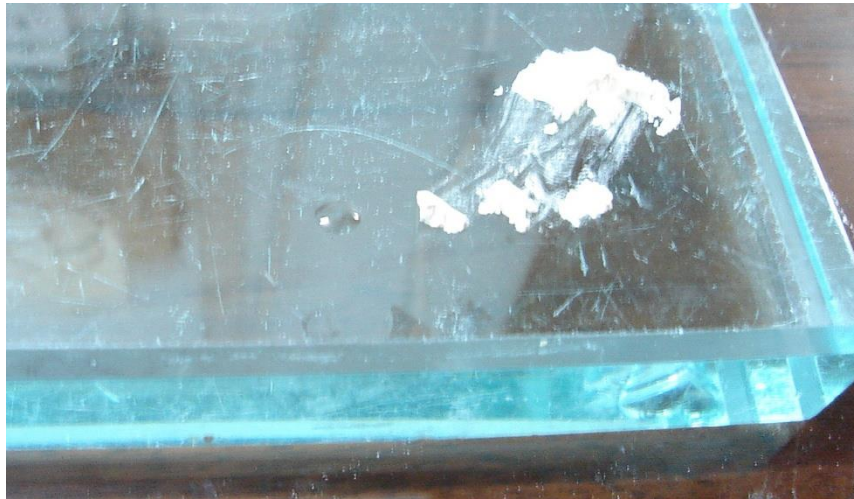
Figure (1). Cement powder divided into small increments on a thick glass slab.
