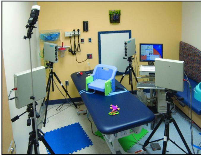
Fig.:An example of a 3D stereophotogrammetry system (3dMDcranial™ System) in a clinical research setting
