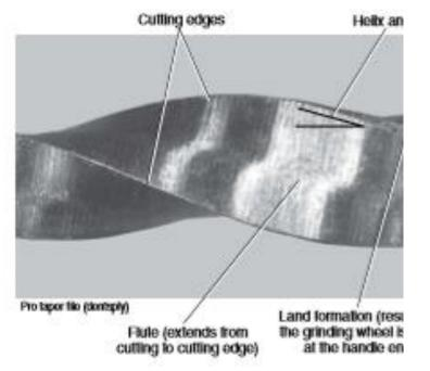
4- If a file is sectioned perpendicular to its long axis, the rake angle is the angle formed by the leading edge and the radius of the file. If the angle formed by the leading edge and the surface to be cut (its tangent) is obtuse, the rake angle is said to be positive or cutting. If the angle formed by the leading edge and the surface to be cut is acute, the rake angle is said to be negative or scraping.
