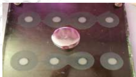
Figure 4: Pressure applied over the cover mold and closure with nuts and G-clamps.
