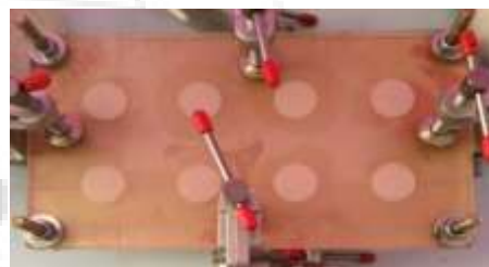
Figure 3: Pressure applied over the cover mold and closure with nuts and G-clamps.
