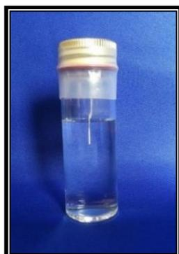
**Figure 1: Immersion of the sample in the artificial saliva.**
