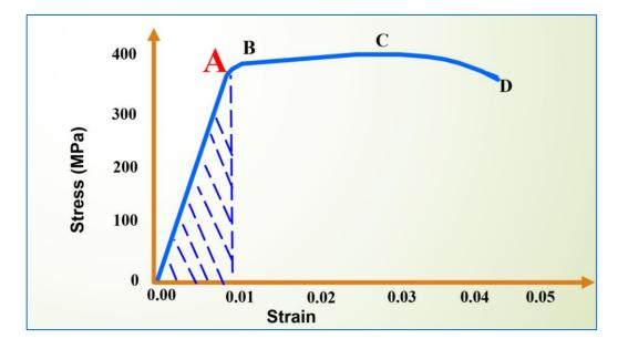
• **<u>Toughness</u>**: It is the total work or energy required to break the material. It's the total area under the stress-strain curve. It requires strength and plasticity.
