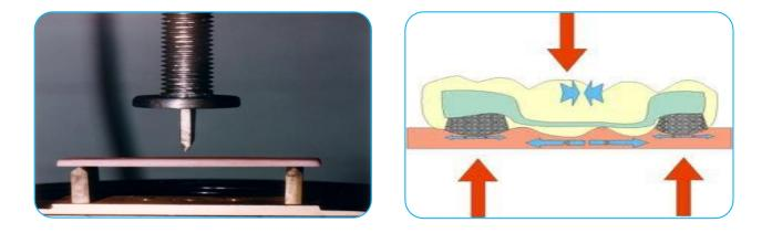
• **Impact strength:** It is the ability of the material to break on sudden impact. Low impact strength means brittle material, like dropping of the denture.
