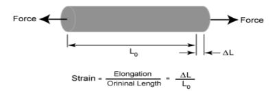
**Strain** (E): is the change in length (dimension) or deformation per unit length (dimension) caused by externally applied force. Strain is denoted as ' $\epsilon$ '. It has no unit of measurement. Examples of some dental materials strain are: acrylic: 1.5%, Co/Cr: 4%, stainless steel: 35%.
