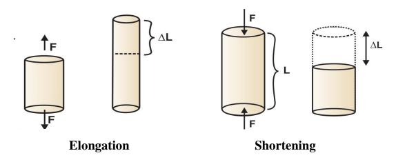
• **Elongation:** The deformation that results from the application of tensile stress. An alloy with high percent of elongation can be bent or adjusted without danger of fracture.  $\frac{\text{Increase in length}}{\text{Original length}} \times 100$
