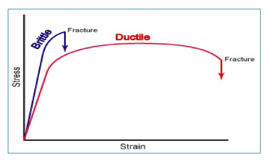
• **<u>Resilience</u>**: The amount of energy absorbed by a structure when it is stressed within the proportional limit. Or it is the energy needed to deform the material to its proportional limit.
