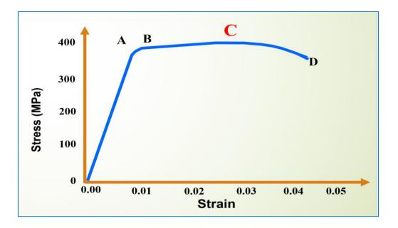
• <u>Fracture Strength</u> (point **D**): The stress at which a material fracture. The fracture strength is not necessarily the ultimate stress at which the material will fracture.
