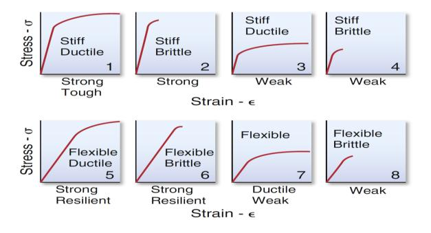
• **<u>Strength</u>**: is the measure of the resistance of the material to the externally applied force.
