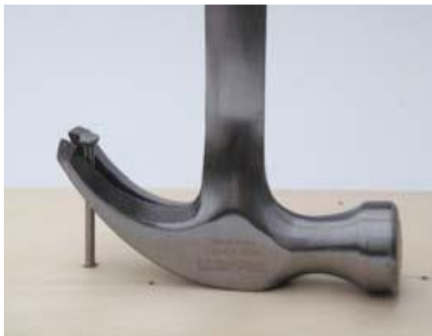
A claw hammer uses class I lever mechanics, with the handle one lever, the head of the hammer as the fulcrum, and the claw as the short lever applied to the nail. The Physics Forceps uses a similar action to remove a tooth.
