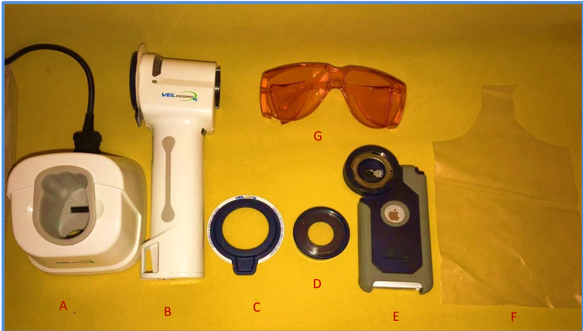
Figure 2.1: VELscope VX component: A. External power brick and power cord, B. VELscope hand piece, C. Protective asepsis anti-fog barrier, D. Protective asepsis anti-fog lens, E. iPod 5 image adaptor, F. Disposable hand piece asepsis barrier, G. Patient safety glasses
