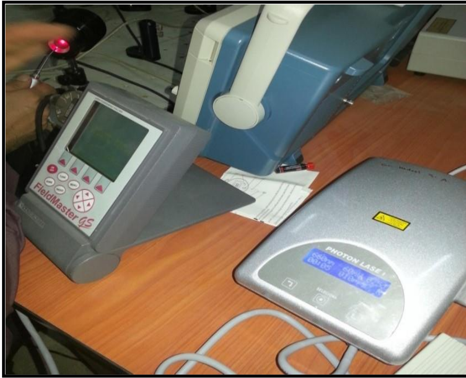
Figure 2.4: Photonlase (IR) laser device calibration.
