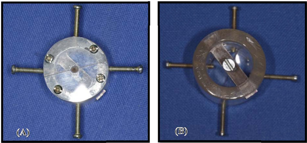
Figure (2-8): The teflon mold. (A) Top view. (B) Bottom view.
