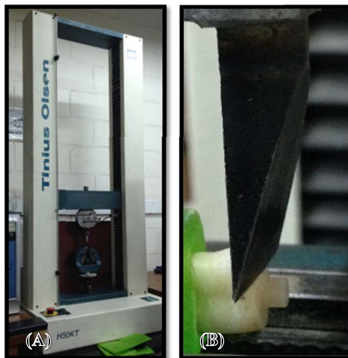
Figure (2-10): (A) Univesal testing machine (B) Sample in lower jaw of the machine.
