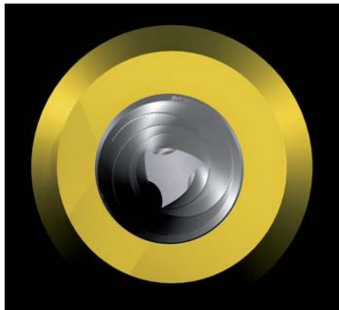
Fig (1-5)WaveOne apical crosssection modified convex triangular.
