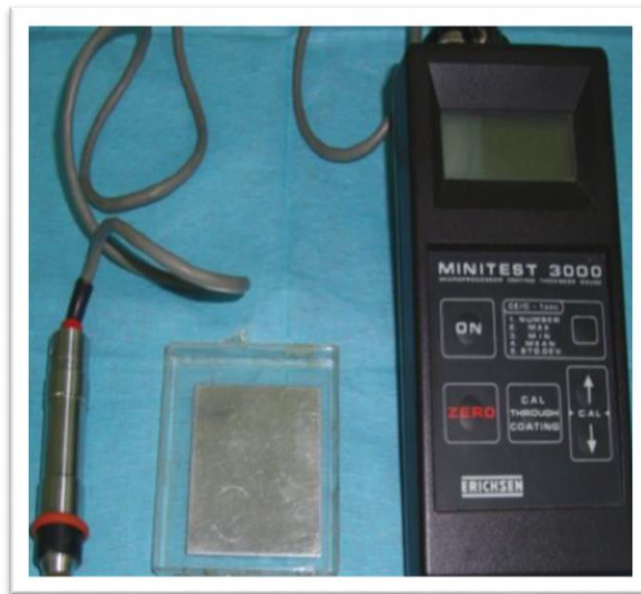
(Figure 2.12): Digital gauge for coating thickness
