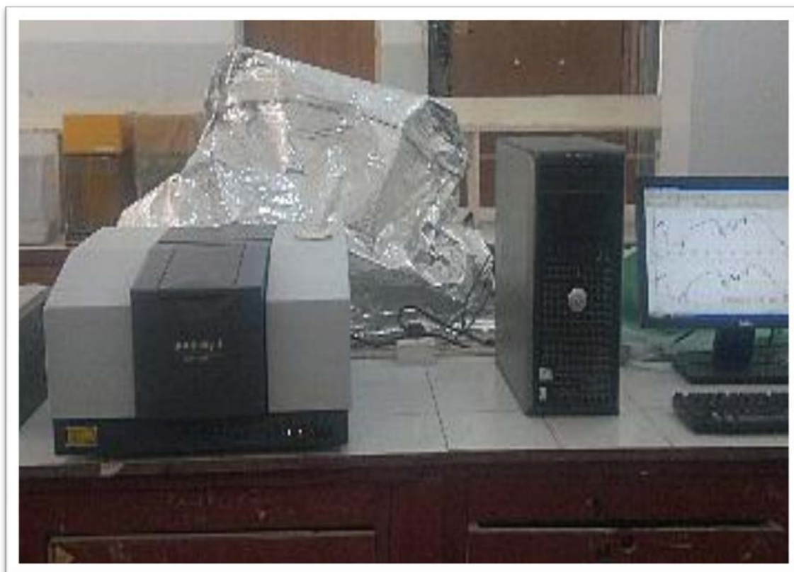
Fig. (2-10): Fourier transform infra –red ( FTIR) spectrophotometer.
