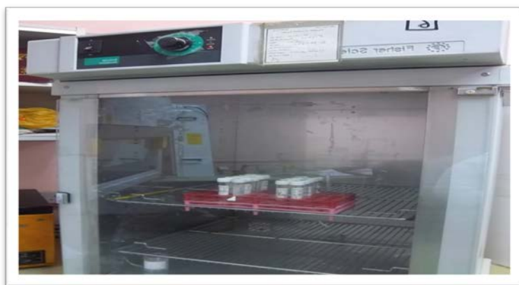
Fig (2-7): Test specimens with artificial saliva in Test tubes under incubation.
