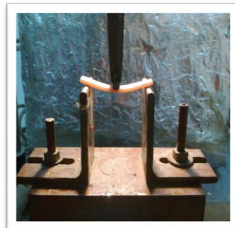
Fig (2-15): A- Instron testing machine, B- Specimen under testing.
