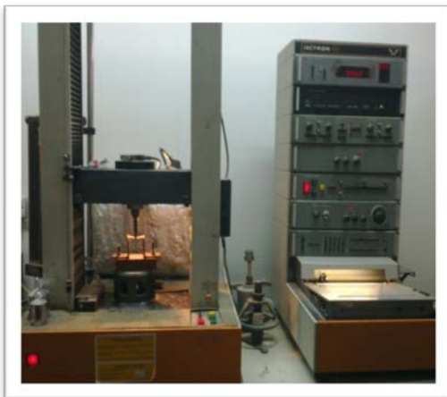
Fig (2-15): A- Instron testing machine, B- Specimen under testing.
