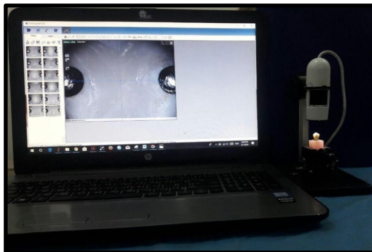
Figure (2.16): Taking images with digital microscope.
