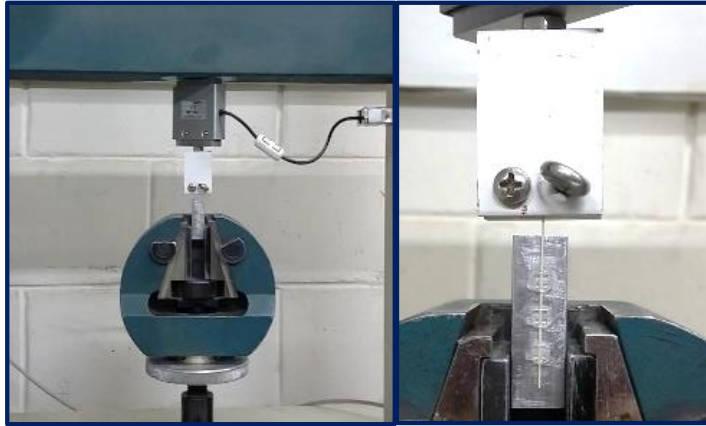
Figure 2.22: Wire-bracket-block system fixed to machine
