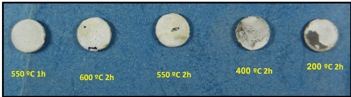
Figure 2.11: Heat treatment at different temperature
