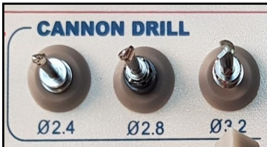
Fig. (2.20): Cannon drill A.I ( \varnothing 3.2 mm) with its edge cutting features and non-traumatic apical end.
