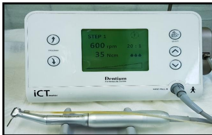
Fig. (2.2): Dental implant engine (Dentium Co., Korea) illustrating settings of the device.
