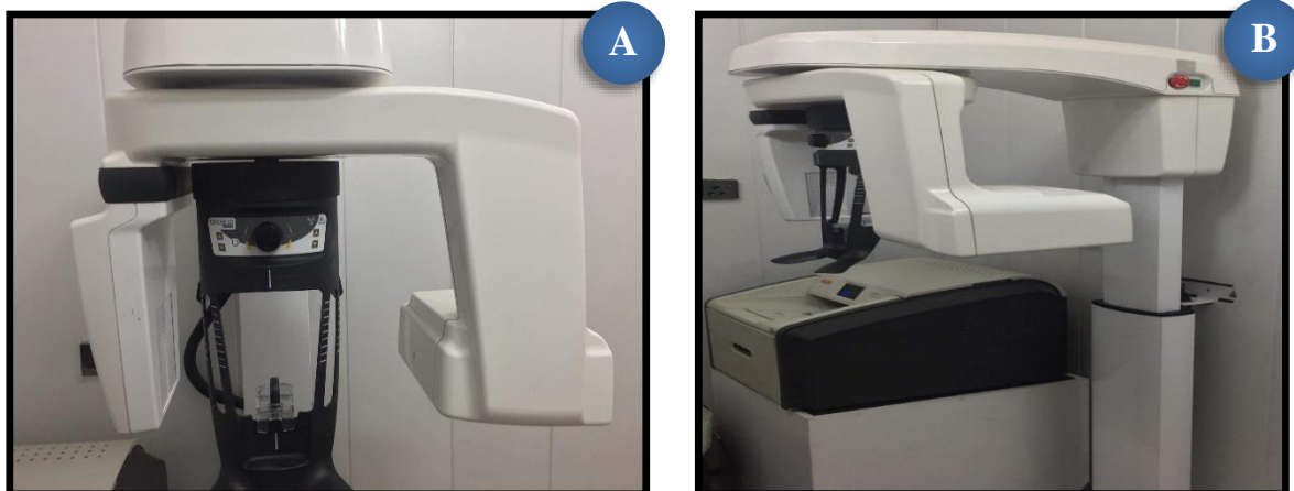
Fig. (2.10): (A) & (B) Kodak 9500 Cone Beam 3D System with effective dose 92 \mu\text{Sv} & Orthopantogram system with effective dose 11.9 (Carestream CS 8100 3D Health Inc., France).
