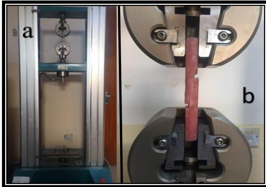
Figure (2-18): a) Instron machine; b) Testing of shear bond strength of soft lining material.
