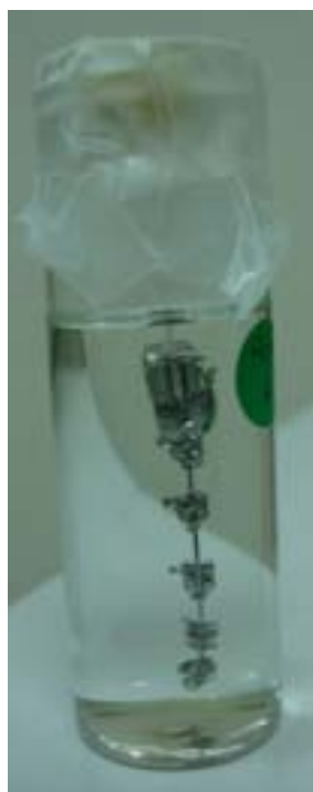
Fig (2–7) Orthodontic Sample Immersed In Testing Solution
