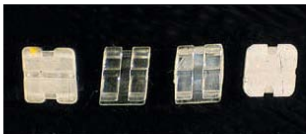
Figure (1–5) Polycrystalline bracket (first, third, and fourth from the left), single crystalline bracket (second from the left) ( Brantley and Eliades, 2001 )
