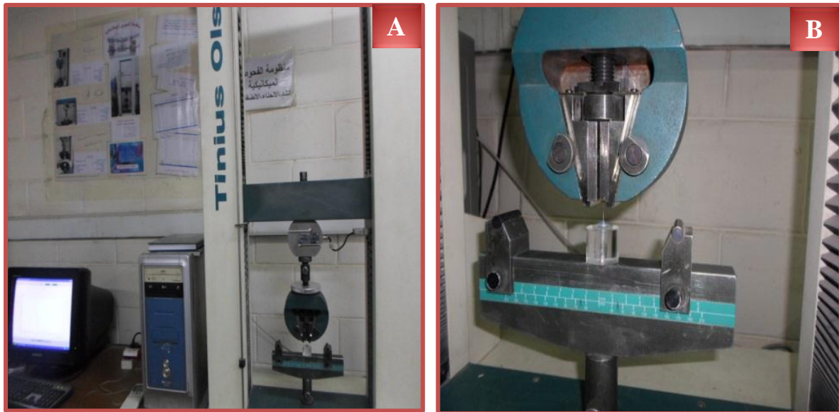
Figure 2.22: Universal testing machine A: Universal testing machine with computer software, B: during push-out test
