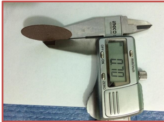
Figure 2.16: Measuring the thickness of the disc with digital caliper
