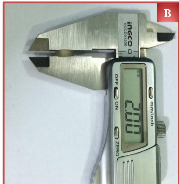
Figure 2.17: Sectioning of the specimen: A: Cutting the specimen with a disc, B: Measuring the specimen with digital caliper
