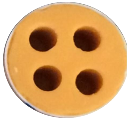
Figure 2.14: Mold made from silicon material
