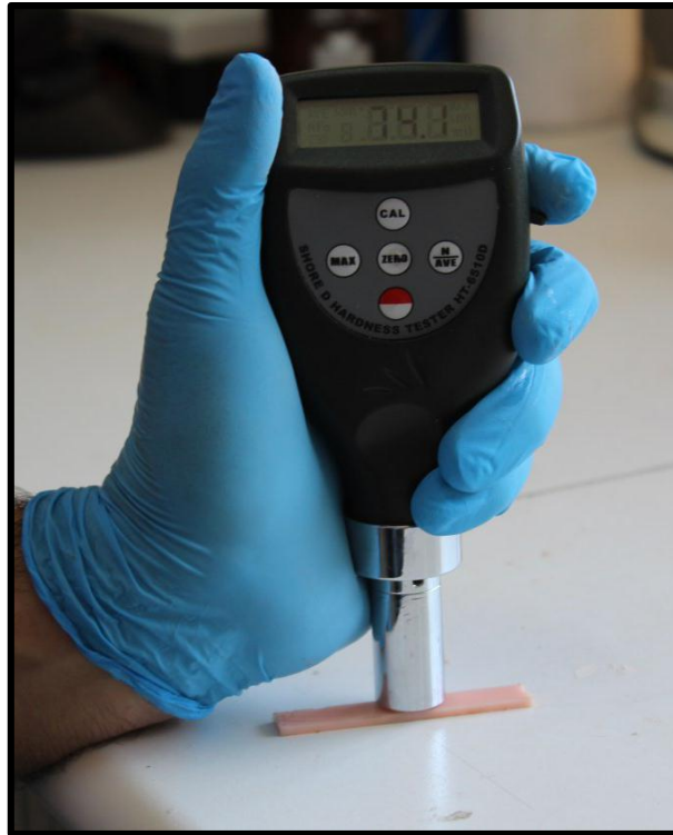
Figure (2.20) Specimen testing with hardness device
