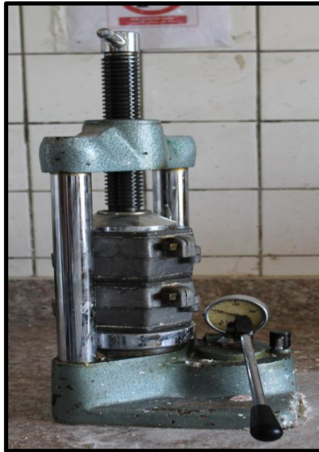
Figure (2.7): Flasks under the pressure of hydraulic press
