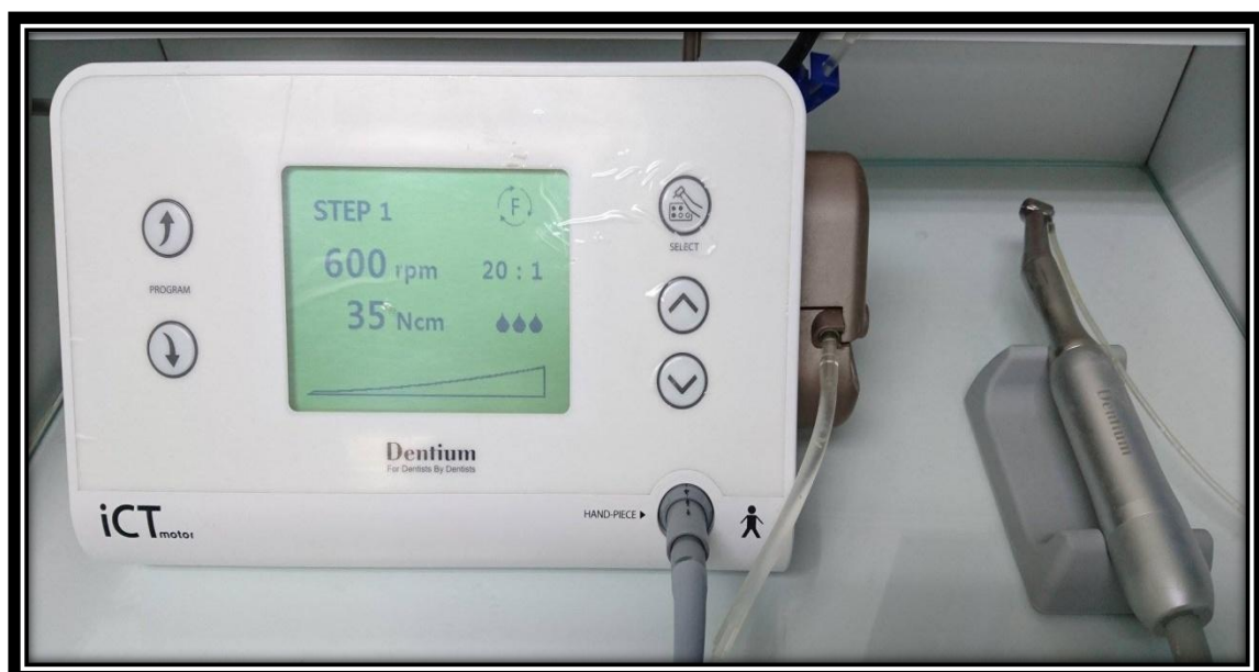
Fig. (2-2): Dental implant engine (Dentium Co., Korea) with settings operated on.
