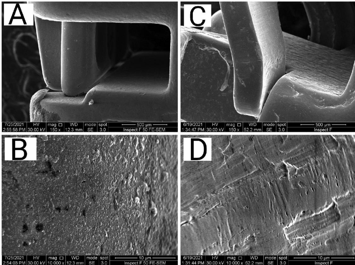
**Supplementary Figure 7:** SEM images of bracket gates before exposure to ageing. A, gate of Damon bracket showing the clip system. B, Damon bracket gate at 10000× magnification depicting score 1, which indicates a relatively flat smooth surface with disperse pits and mild surface irregularities. C, clip design of Pactive bracket gate. D, Pactive bracket gate at 10000× magnification eliciting score 2, which identifies a relatively rough surface with pits and scratches.
