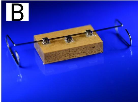
**Supplementary Figure 1:** A, an experimental block with 3 squares, setting the central one 2 mm higher than the others. B, aligning the brackets on the plastic block using a straight stainless steel wire of 0.021\*0.025" gauge.
