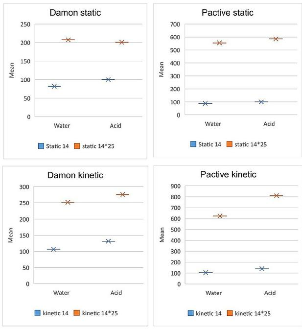
**Supplementary Figure 4:** Descriptive statistics of the static and kinetic frictional forces (g) of 4 subgroups. Pactive brackets demonstrated higher mean values than Damon brackets post both ageing conditions.
