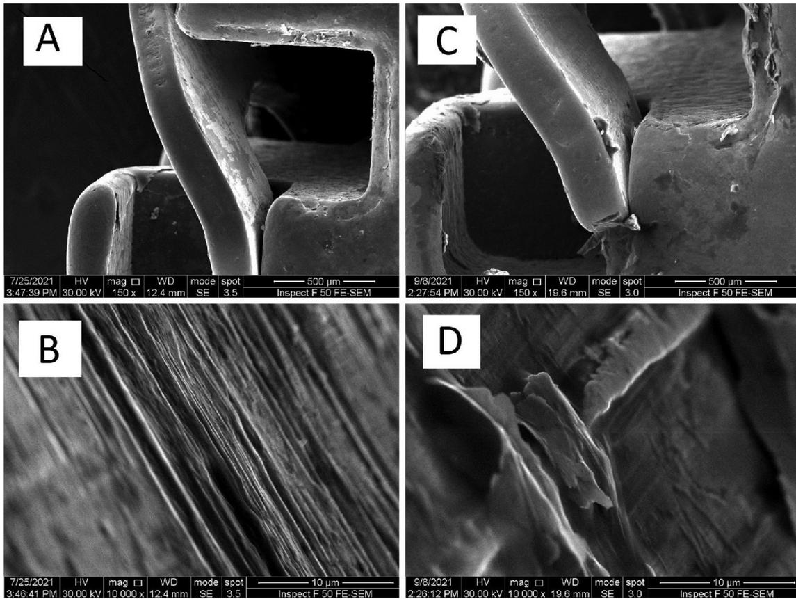
**Supplementary Figure 9:** SEM images of Pactive brackets gates post exposure to ageing conditions; A: Pactive bracket gate after water storage, B: at a higher magnification (10000×) the gate surface demonstrates score 2 after water storage, C: Pactive bracket gate after acid challenge, D: at a higher magnification (10000×) the gate surface depicts a rough surface with pits, scratches/grooves and marked surface irregularities (score 3) after acid challenge.
