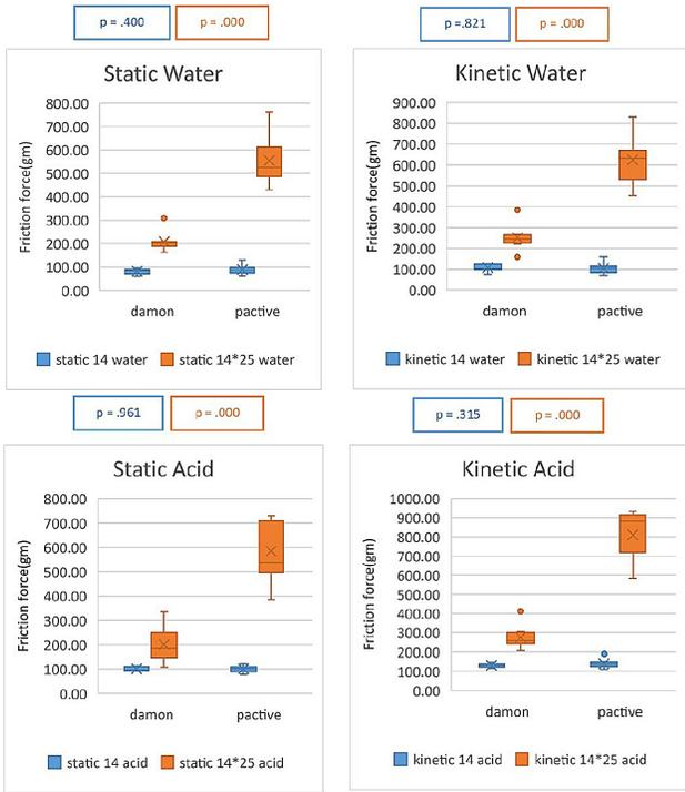
**Supplementary Figure 5:** Independent t-test for the comparison of frictional forces between the two bracket systems showing non-significant differences when using round CuNiTi wires, while Pactive system yielded significantly higher frictional forces than Damon system when coupled with the rectangular CuNiTi wires.
