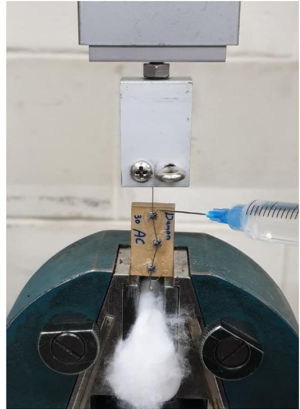
**Supplementary Figure 3:** friction test using the Instron machine, showing dripping of distilled water from a plastic syringe during the test.
