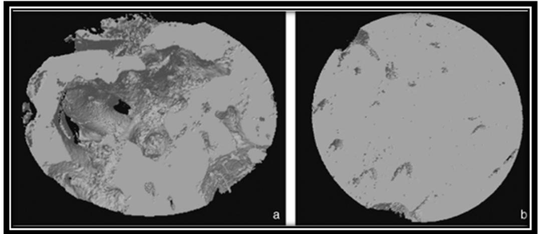
**Figure 1.5:** 3D axial images of bone cores. Despite the sample (a) being less dense than sample (b), possibly it has a rod/sphere-like pattern of the trabeculae, higher surface area and therefore, a greater BS/BV(Gomes de Oliveira *et al.*, 2012).
