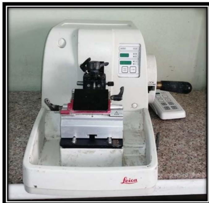
**Figure 2.10:** Microtome (Leica, Germany).
