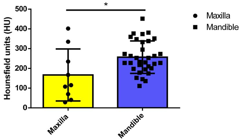
**Figure 3.1:** Scatter plot with bar graph showing the difference between the bone density (HU) of the maxillary and mandibular proposed DI sites measured by CBCT (P=0.0148).
