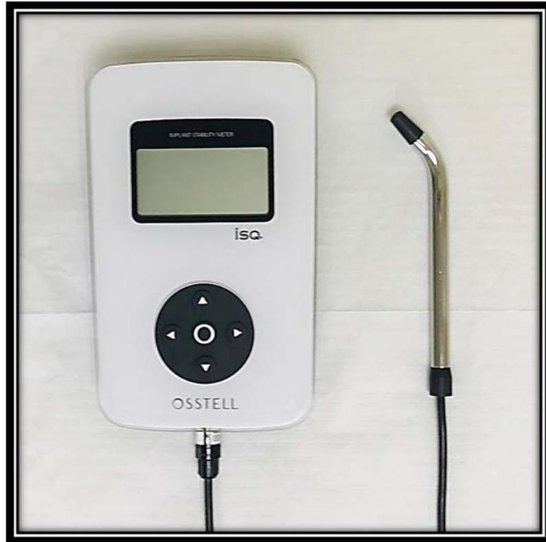
**Figure 2.7:** Osstell® ISQ device for measuring implant stability (Osstell®, Gothenburg, Sweden).
