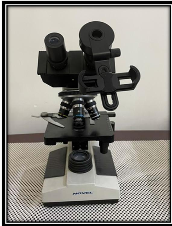
**Figure 2.11:** Optical microscopic with a smart phone adapter (Novel, China).
