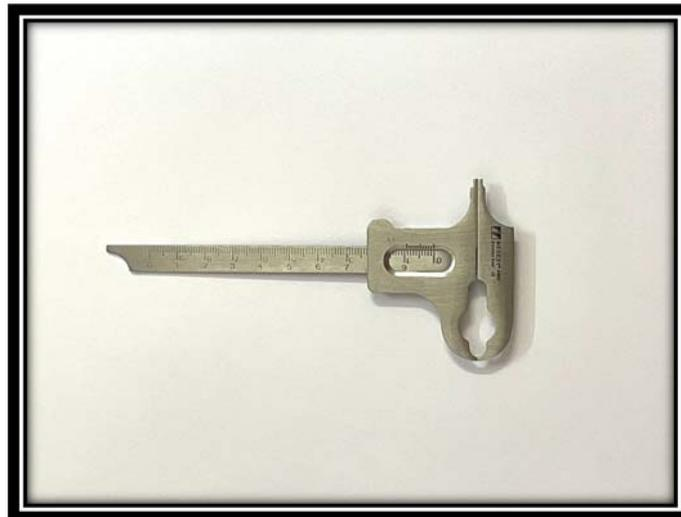
**Figure 2.6:** Vernier caliper for preoperative space analysis (Stainless hardened steel, China).
