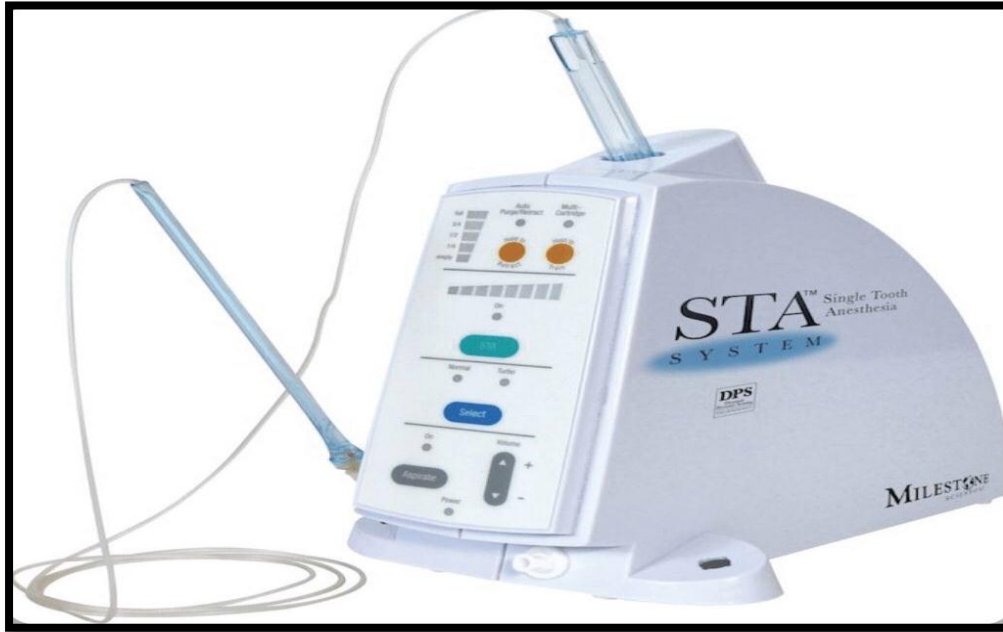
Fig.19 Computer controlled local anesthesia delivery system with dynamic pressure sensing (Veneva et al. , 2018).
