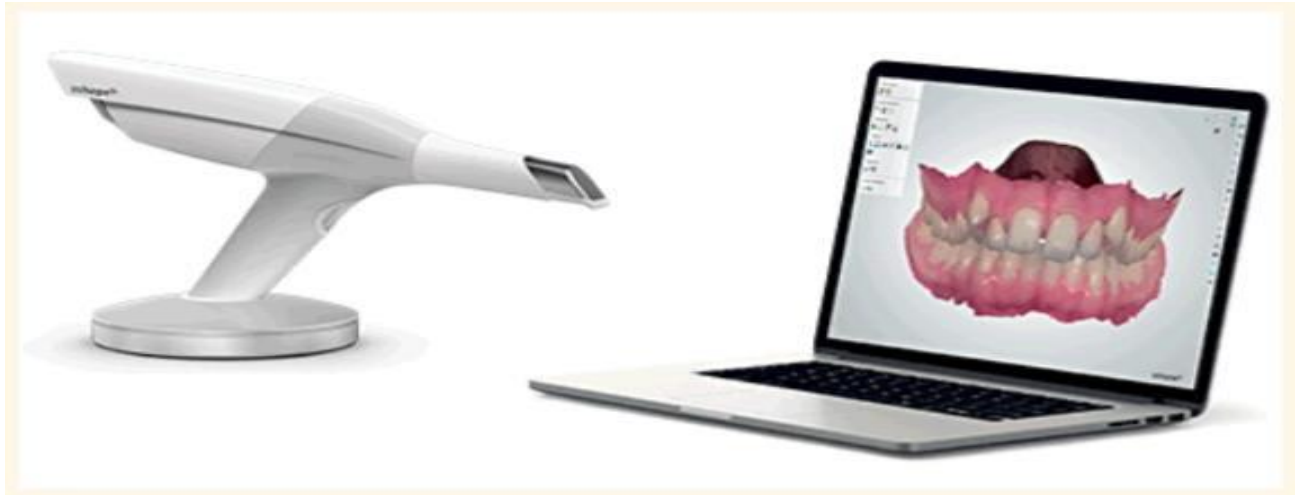
figure 3 : scans the geometry intra orally and send it into the computer
