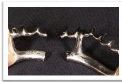
Figure (1.6): Fractured connector. ( Aditama and Sabdayana, 2019 ).
