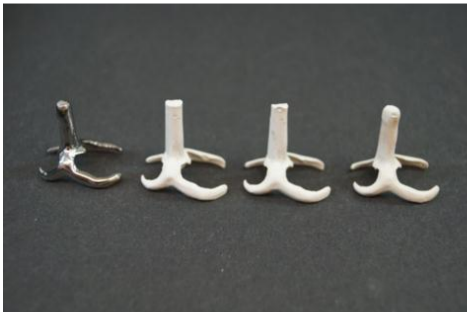
Figure 4: RDP clasp specimens made of CoCrMo, PEEKmilled1, PEEKmilled2, and PEEKpressed
