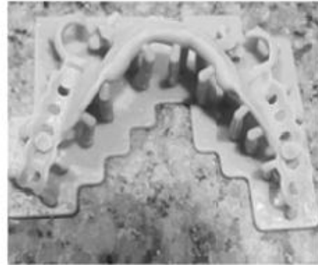
Figure 12: Resin pattern of the framework made with prototyping technology
