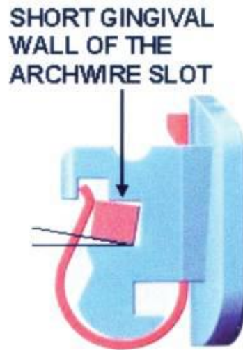
Figure 7: Diagram of a SPEED bracket with rectangular wire showing the reduced gingival slot wall depth and consequent reduction in torquing ability (Haraddine, 2003).
