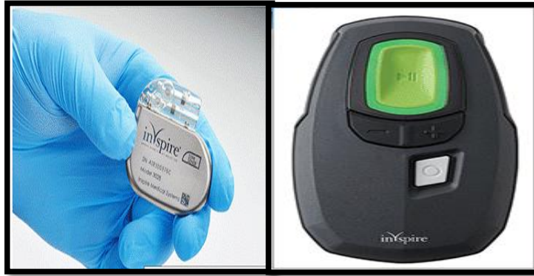
Figure8: Inspire Upper airway electrical stimulation system, Implantable device(left), remote(right). (Inspire Medical Systems, 2020)
