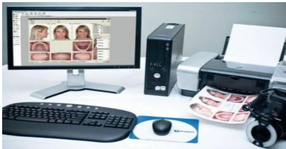
Fig. 1.11 Modern digital imaging system includes a digital camera, a computer, a colour printer and an image management software ( Karad, 2010 ).
