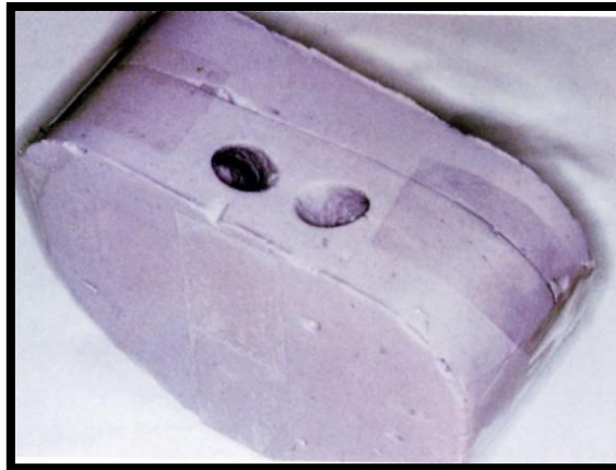
Figure (1-2e) Sprue holes are then cut into the posterior border of the alginate mold.
