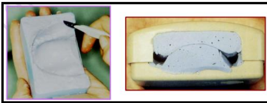
Figure (1-3g,h) Two halves are then opened and the sprue holes are cut with a Sharp knife. The halves are then re-assembled and can be held together with elastic bands.
