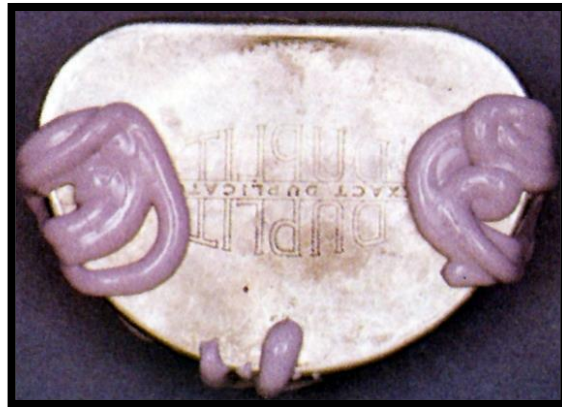
Figure(1-2c) The flask is then filled with a new mix of alginate - avoiding any air entr-apment, and the lid is closed.
