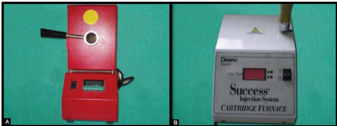
Figure 1.11 A and B electric cartridge furnace (Singh and Gupta,2012).
