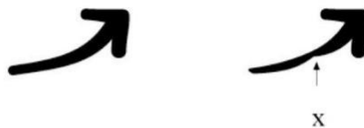
Figure 3.3 A narrowing of the clasp arm creates a point of flexure which weakens and affects the flexibility of the clasp, since flexure begins at this point ( Loney,2011 ).
