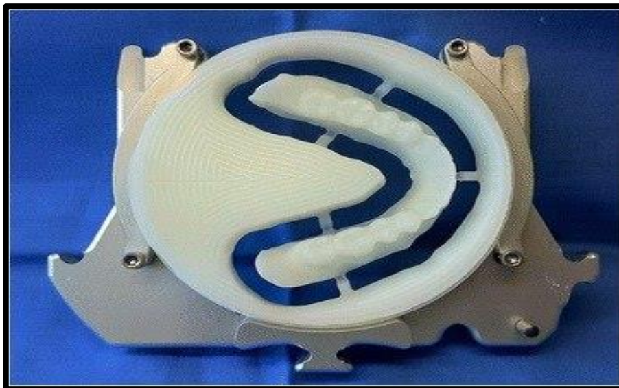
Figure 1.14: Manufactured template on a white PMMA disc (Bonnet et al. ,2017).
