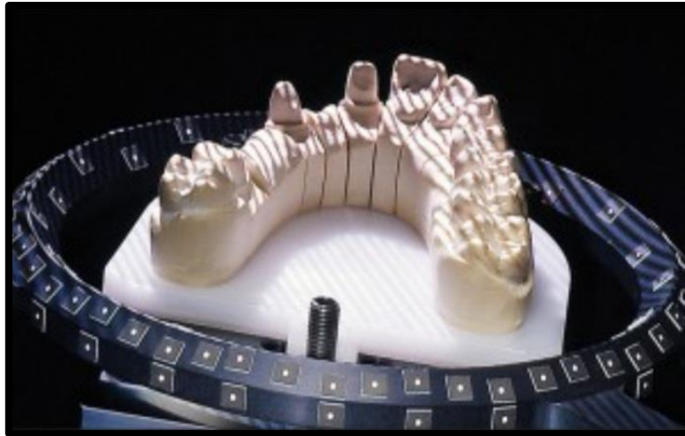
Figure 1.2: LED Based scanner.
