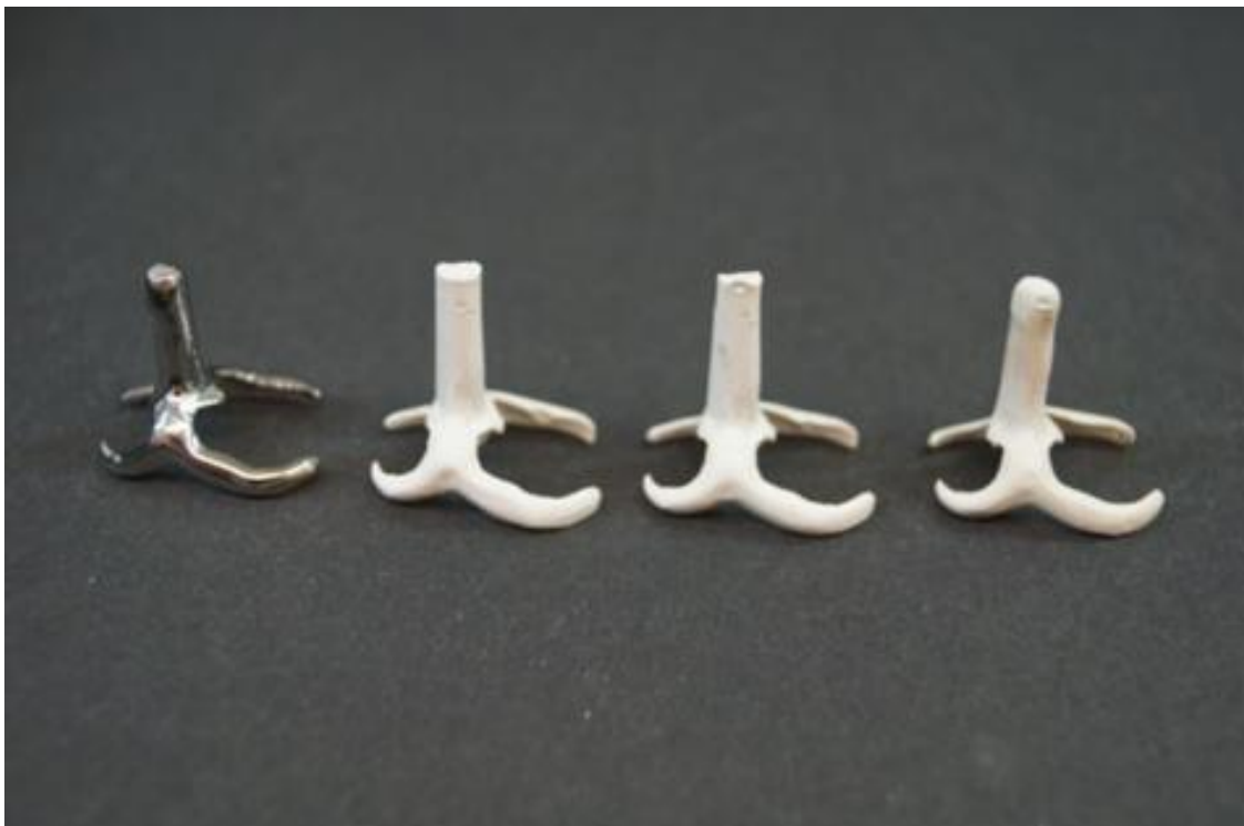
Fig. 2 RDP clasp specimens made of CoCrMo, PEEKmilled1, PEEKmilled2, and PEEKpressed. ( Gao et al. , 2015 ).
