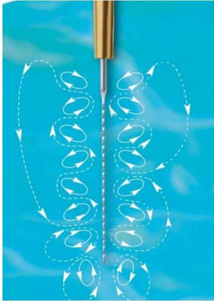
Fig.No.14 :Depiction of the waves generated around the vibrating ultrasonic file
