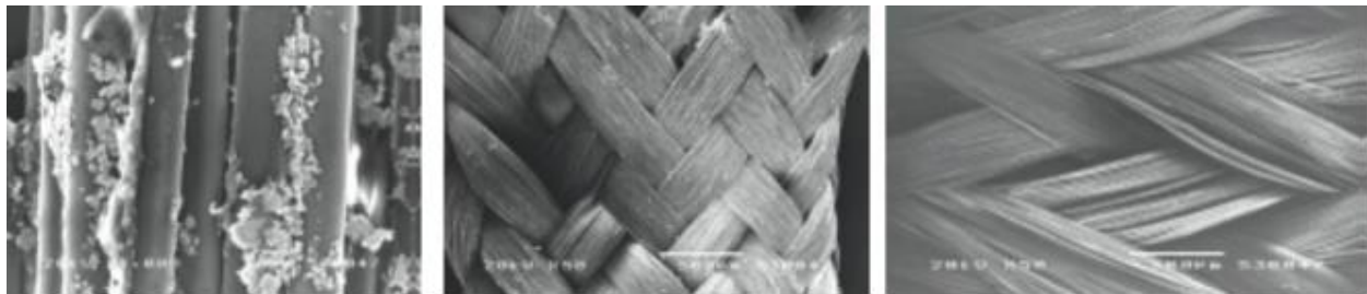
Figure (2): Scanning electron micrographs showing the different architecture of fibers available for dental use. (left to right): Unidirectional and pre-impregnated); Glass span (woven in rope manner); Connect (woven)
