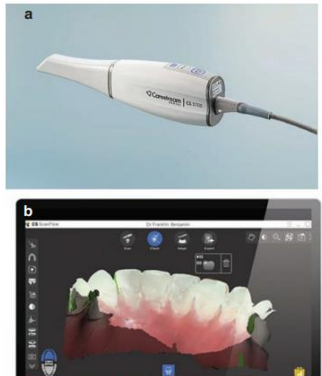
Figure 12: (a) Carestream CS 3700® automatically detects the enamel color of the scan area to help identify the correct position for restorative outcomes (Adapted from Carestream Dental LLC). (b) Intraoral imaging of Carestream CS 3700®
