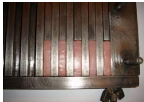
Figure 1: Metal mould of denture base specimens for tensile testing
